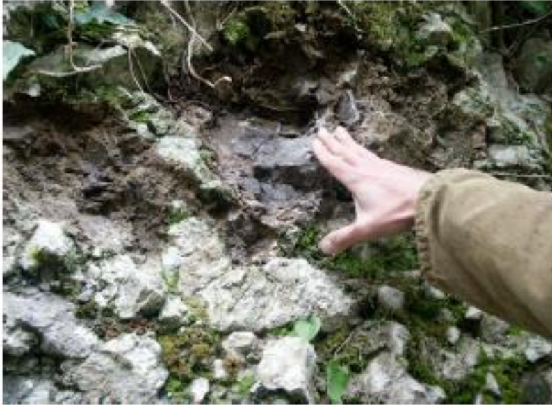
Figure CS10B. Brecciated limestone filled by bitumen.
