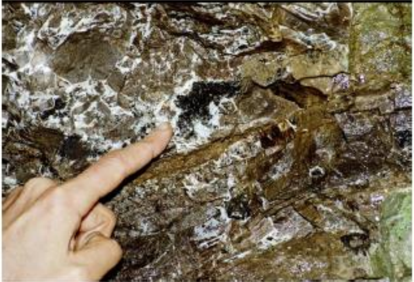
Figure CS11F. Brecciated limestones firstly were filled by calcite and then by asphalt (oil)
