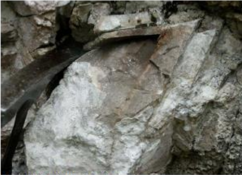
Figure CS12B. Fresh chip of the bituminous limestone.
