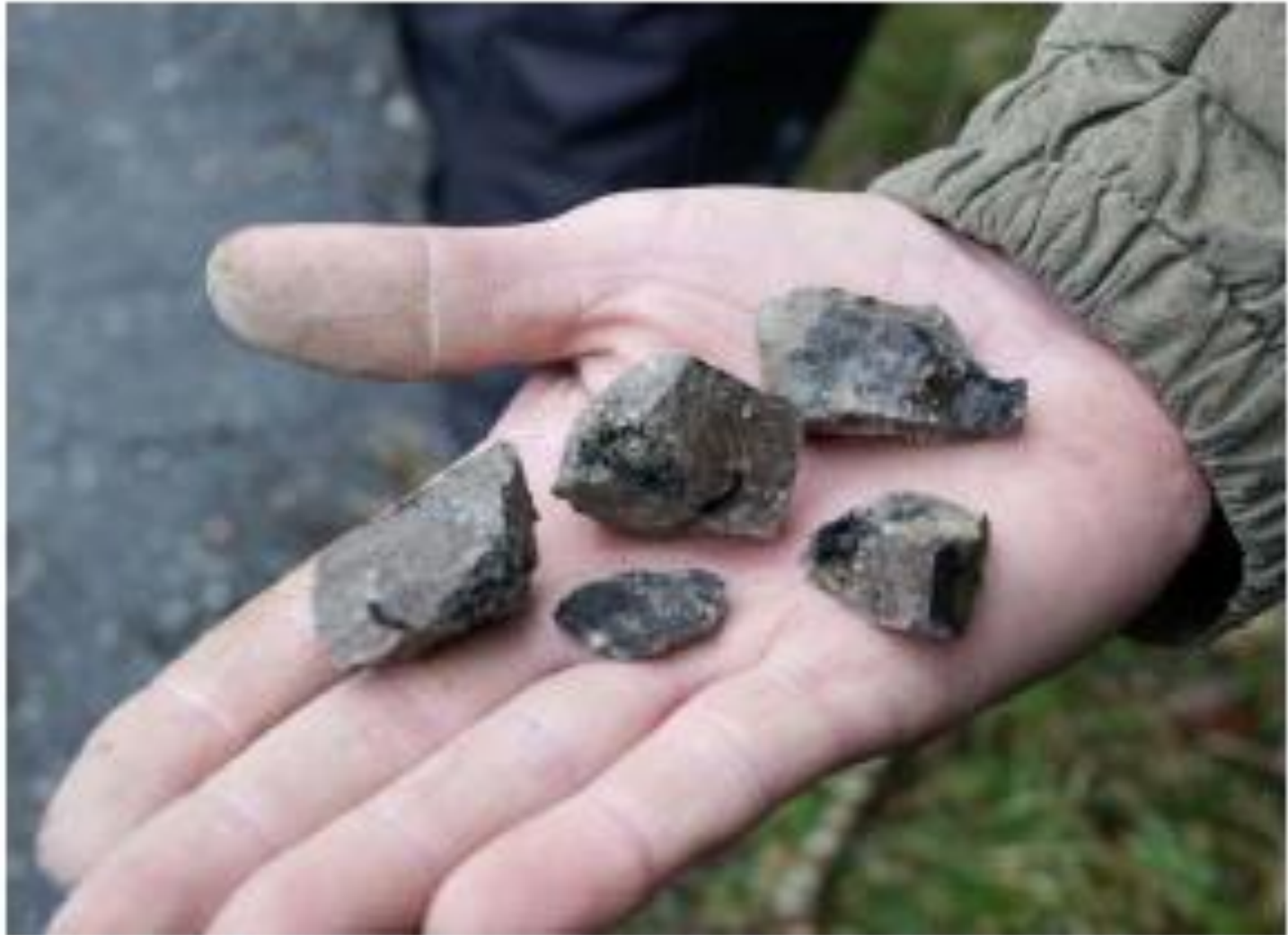
Figure CS10F. Spots of bitumen inside a rock.
