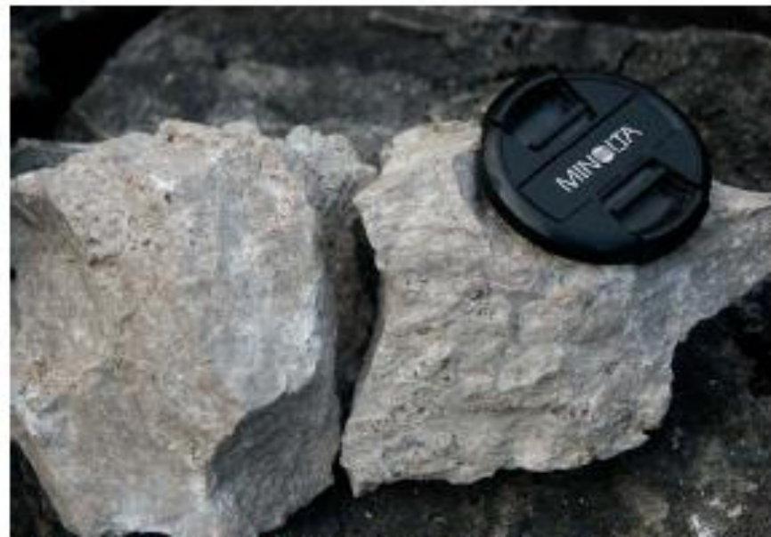
Figure CS7B. Strongly poriferous limestone having a distinct gas smell.
